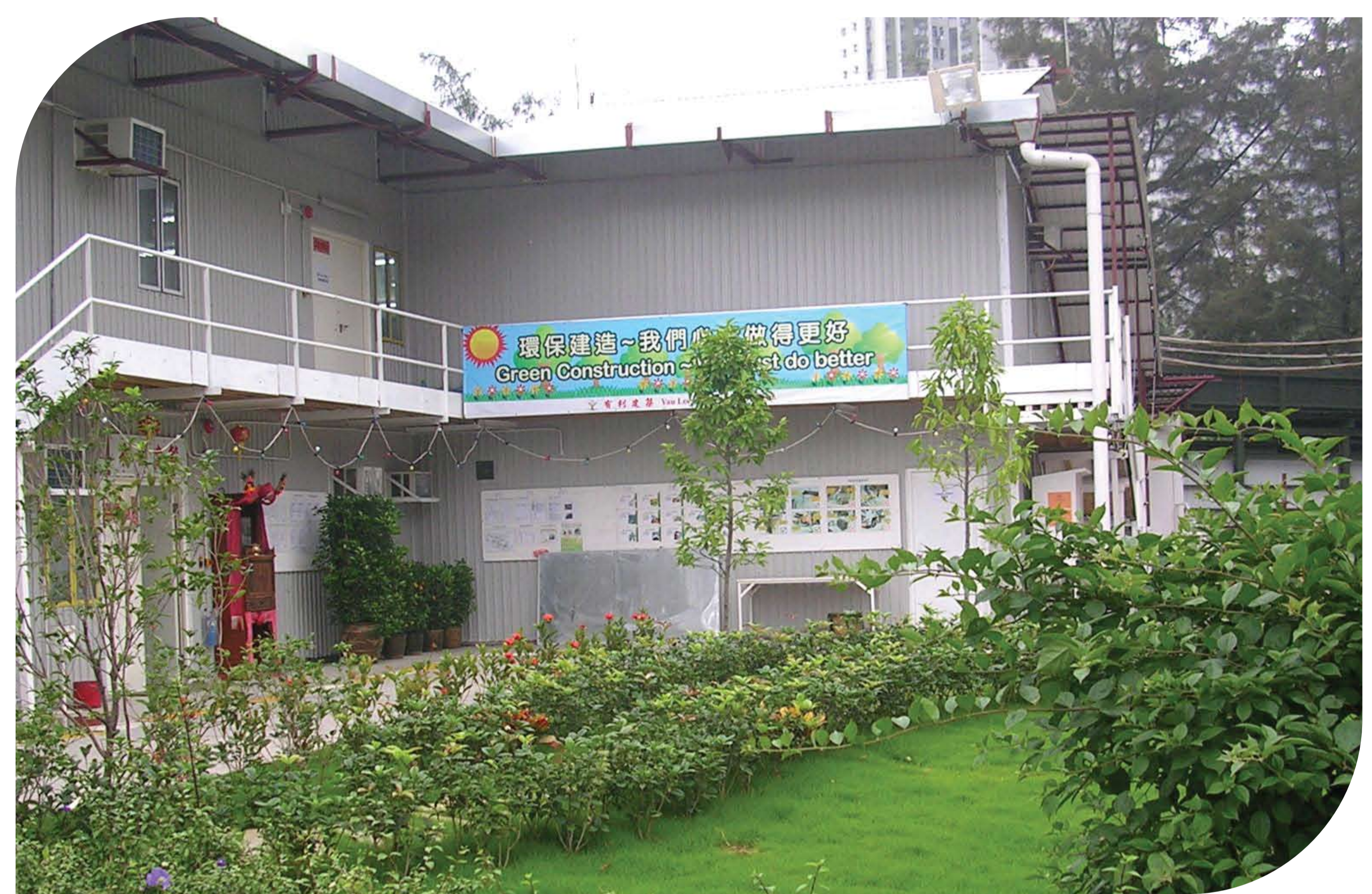
組裝式地盤臨時設施 Site Office with Reusable Structural Steel
