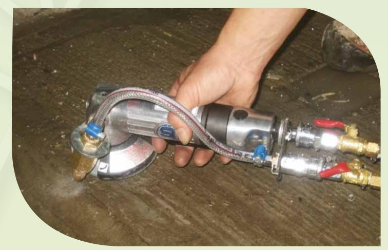
研發無塵磨機,減少施工時所造成的灰塵。 We invented the Dust-free Grinding Component to eliminate dust during concrete grinding.
