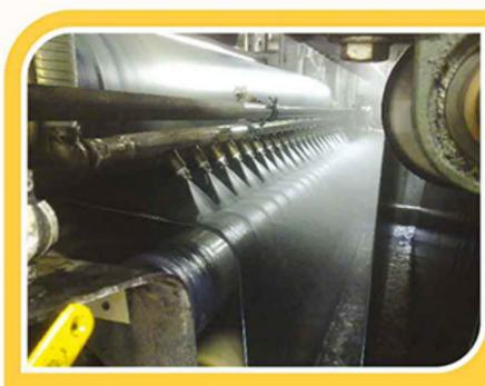
改良噴水設備節省用水。 Water sprays alterations to reduce water consumption.
