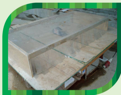
鋸床加設創意環保蓋以控制塵埃 Circular saw equipped with innovative cover on the bench for dust suppression
