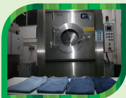
G2無水漂洗系統使牛仔褲漂洗工序實現了「無水、無藥」 G2 Waterless Bleaching System - "No-water-or-chemical" for denim jeans manufacturing
