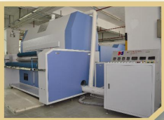
蒸汽預縮機由公司自行研發(待批專利)，使噴水、烘乾、預縮及攤布的程序一體化，實得高效節水、節氣。 Steam pre-treating machine, an in-house designed and developed (pending patent) all-in-one machine for spraying, drying, pre-shrinking and spreading, highly reduces water and steam consumption.
