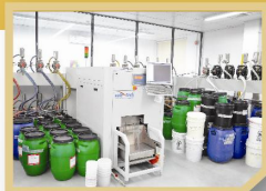
自動調膠機的配膠準確性高，能減少膠料浪費和污染。 Automatic ink dispenser is accurate in blending dyes and paints, thus reducing wastage and pollution.
