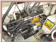
注塑機伺服系統節能改造項目，節約能源及降低噪音。 HEs servo system for injecting mold is modified to save energy and reduce noise.
