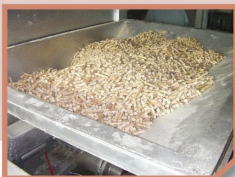
採用生物顆粒燃料替代柴油燃料，節能效率達66%。 Diesel oil was replaced by biological granular, saving 66% of energy.
