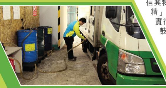
貨車採用B5生物柴油,並設置生物柴油加油站。 Using biodiesel (B5) for trucks and setting up a biodiesel filling point.
