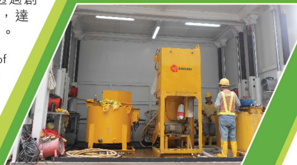
利用循環再用的貨櫃及廢鋼建造「組合式灌漿台」平台。 Building "Modular Grouting Platform" with recycled containers and scrap steels.
