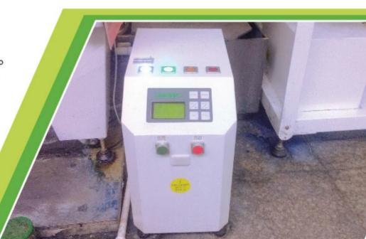
安裝智能顯影液循環補充系統和沖版廢液處理設備,減少使用化學品。 Installing developer filtration and recycling system to reduce chemicals consumption.
